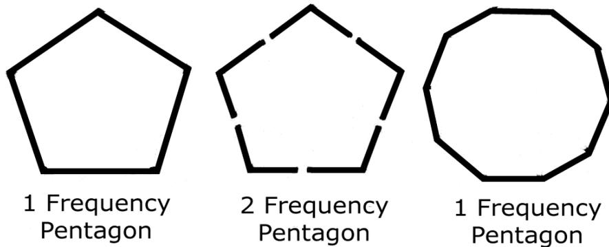
The five struts of a pentagon in the original wave become the 10 struts of the decagon as the symmetry shifts. The above diagram of the 'equator' of a 6-pentagonal tensegrity sphere illustrates this shift. When a pentagon goes from 1-wave number to 2-wave number, its edges double to become a decagon. We now have a 6-decagonal tensegrity sphere in which we have changed both angle and wave number.
